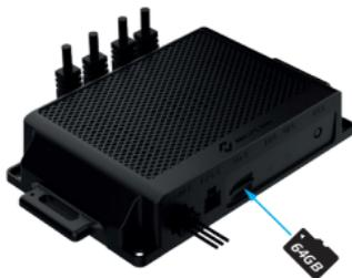
Card removal: carefully press the card and remove from the slot.
